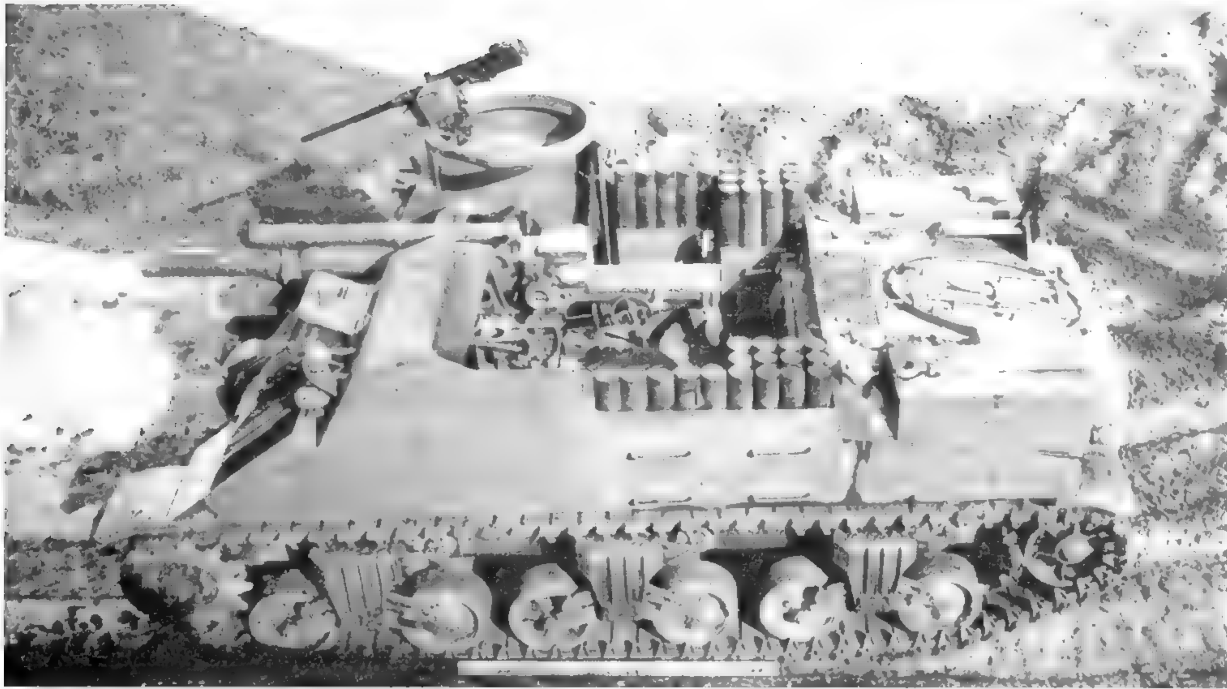
The cylinders arranged around the perimeter of the open-topped fighting compartment of the M7 contain 105mm ammunition. In this photo the driver's vision hatch is open to provide a clear view as the vehicle prepares to tackle the hill climb test at Aberdeen Proving Ground. This is the first vehicle assembled by American Locomotive Company. (U.S. Army photo)
